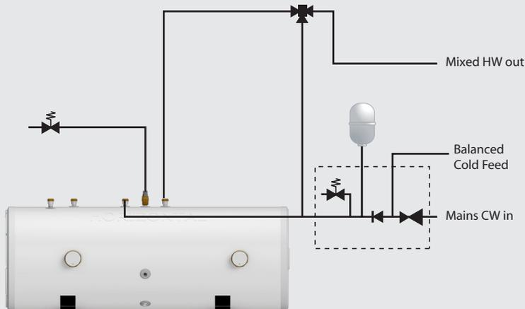
Figure 2 shows the cold water port of the blending valve connected to the balanced cold water outlet. This arrangement will only be acceptable if a WRAS approved non-return valve is fitted, otherwise: -
