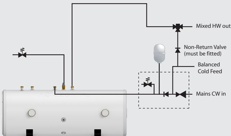
Figure 1 shows the cold water port of the blending valve connected to the mains cold water supply before the inlet control group. This arrangement is completely unacceptable and illegal because: -
