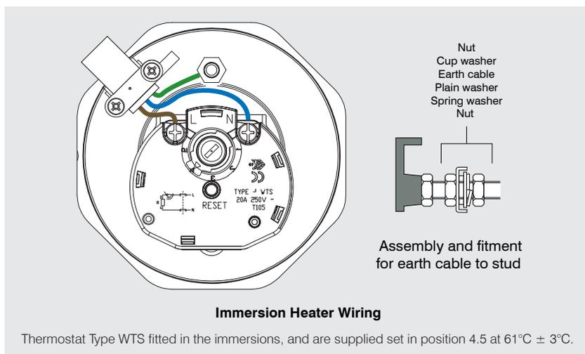
The immersion heaters fitted to our units are 3kW 240V ~AC. Check that the mains supply conforms to this, and all external wiring conforms to the most recent revision of the IEE wiring regulations. An Incoloy element is used on this product for standard domestic use and water conditions.
