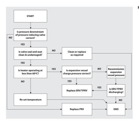
**FAULT - Water Discharge Into Tundish**
