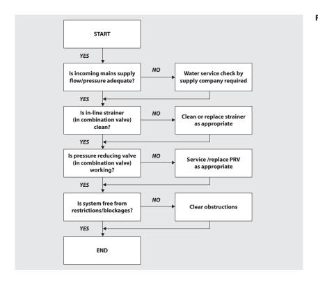
**FAULT - Poor Water Flow at Hot Taps**
