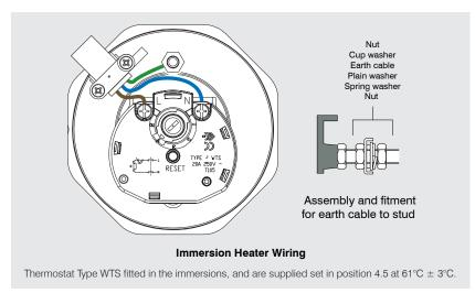
The immersion heaters fitted to our units are  $3kW\ 240V\ \sim AC$ . Check that the mains supply conforms to this, and all external wiring conforms to the most recent revision of the IEE wiring regulations. An Incoloy element is used on this product for standard domestic use and water conditions.
